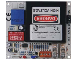
> P/N: H19004300. Hipot Testing Option Kit (1500VDC 10mA)
